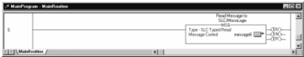
Figure 7.12 Example of a read MSG instruction from a Logix5550 to a SLC or MicroLogix controller
