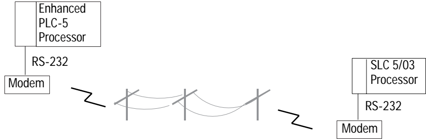
Figure 10.2 Use the public switched telephone network to communicate between a master station and multiple remote stations.
