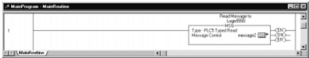
Figure 7.8 Example of a read MSG from a Logix5550 to a Logix5550 controller
