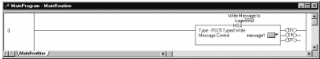
Figure 7.7 Example of a write MSG from a Logix5550 to a Logix5550 controller
